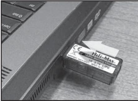
❑ Plug the USB charger into your USB port. The *power indicator light* on the charger will illuminate red indicating that the charger is ready for use.
