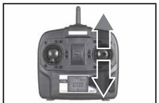
Moving the **cyclic stick forward or backward** will cause the helicopter to tilt and start moving that direction.
