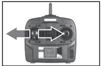
Moving the **tail rotor stick left or right** will cause the helicopter nose to rotate in that direction.
