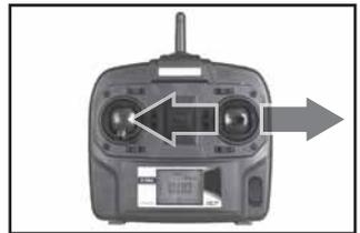
Moving the **cyclic stick right or left** will cause the helicopter to tilt and start moving that direction.
