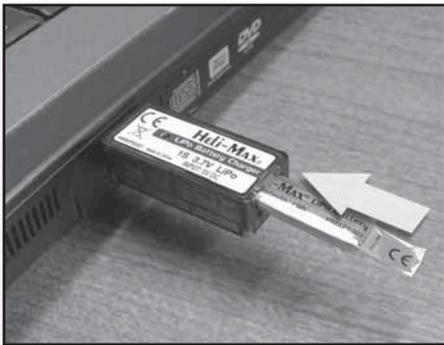
❑ Plug the battery into the charger. The indicator light will start flashing, indicating that the battery is being charged. Once the battery is completely charged, the charge indicator light will stop flashing. Disconnect the battery from the charger. Under normal operating conditions, the battery may take up to 60 minutes to recharge.
